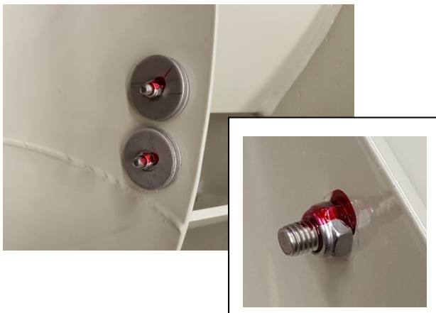
Figure: Basic principle: Secure the balancing weights with coloured marking ink (Loctite SF 7400, or SF 7240 thread-locking varnish).
